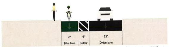
This cross section is recommended for 11th Street on the north side and the west side of the triangle at 12th Street, viewed here looking east (above the triangle) and north (west of the triangle).
