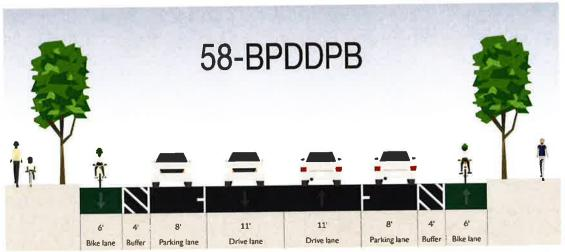
This cross section is used on 10th Street (between Boulder and Detroit Avenues) where the cartpath widens to 58 feet, allowing for the addition of a second flank of parking to the south side.
