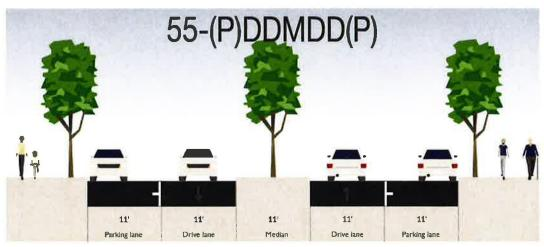
This cross section is recommended for Denver Avenue between 1<sup>st</sup> and 7<sup>th</sup> Streets, viewed here looking north. As the cartpath varies in width between 55 and 57 feet, the median would vary correspondingly between 11 and 13 feet. If a median cannot be built soon, it should be striped in anticipation.
