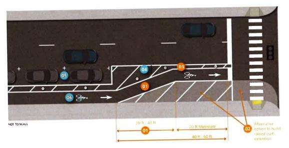
An illustration of how to angle a bike lane around a curb extension with minimal loss of parking spaces. Source: Federal Highway Administration's Separated Bike Lane Planning and Design Guide, p110.
